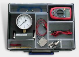
Calibration kit for calibrating pressure and temperature. The kit contains: 1 pressure gauge, 1 multimeter, 1 set of resistors, 1 set of test leads, 1 trimmer, 1 mini screwdriver.
